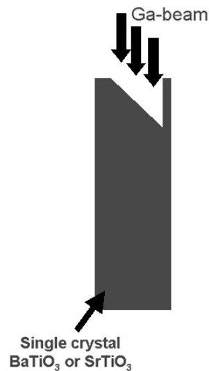
Figure 7. Focused-ion beam production of ultra-thin ( d = 70 nm) single crystal ferroelectric (Saad et al 2004).
